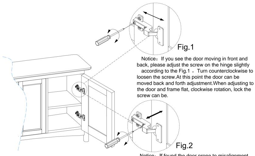
Notice: If found the door prone to misalignment, please adjust the screw on the hinge slightly according to the Fig.2, to make door is in alignment. Gaps between door and post become bigger when clockwise switch, otherwise smaller when counter clockwise.
